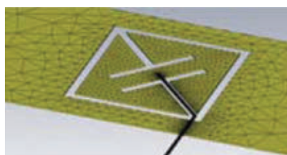
▲ Fig. 6 Metamaterial RLC resonator. 7
